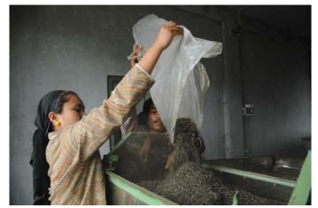
for processing raw tea leaves produced by the tea growers of Mawlyngot village as well as neighbouring villages like Jatah Nonglyer, Mawsna, etc. The society started the tea processing unit as a pilot project with a small capacity rolling table, and indigenous equipment like the withering trough and a drying machine. This unit
